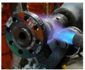
than 50% efficient. *Hot Coils®* induction heating system is close to 95% efficient. This means that more energy is transferred directly to the area to be heated resulting in quicker more accurate heating of the joint.
