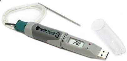
This standalone data logger measures and stores up to 32,510 temperature readings from either a K, J or T type thermocouple.
