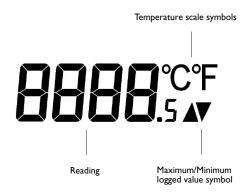
Three different functions are available on the display – most recent logged temperature, maximum logged temperature and minimum logged temperature. The push button is used to cycle through the functions. In addition, logging and alarm status are shown using two high intensity LEDs.
